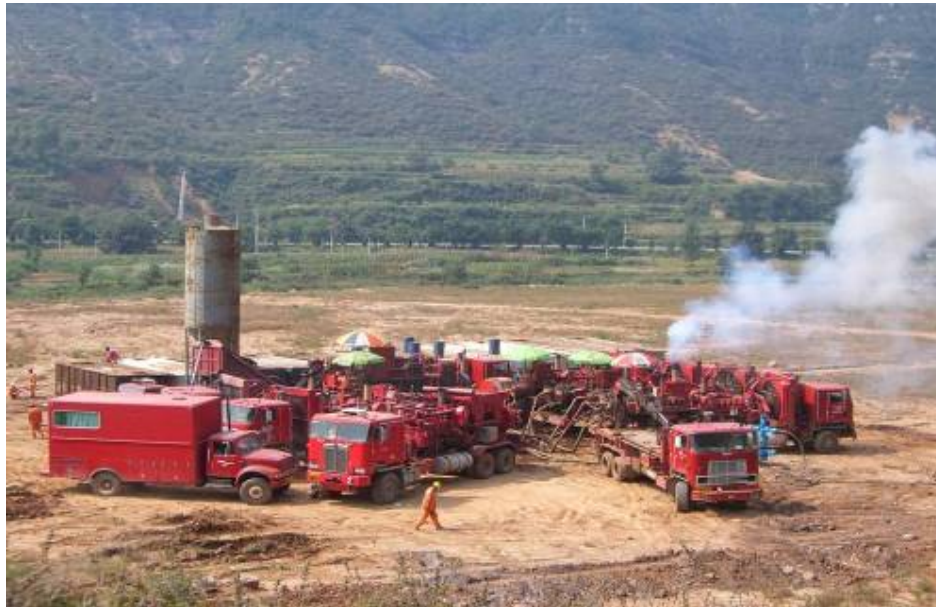
CBM field fracturing
